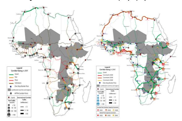
Figure 5. ARTIN Corridor Condition in 2009 and Capacity Gaps by 2040
