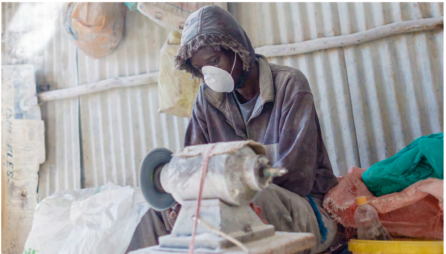
At Victorious Bones Crafts, Dennis Ojala is softening and cutting bones into different shapes and sizes. This process produces a lot of white dust which is harmful to the lungs. Photo: Brian Otieno, Storitellah.com
